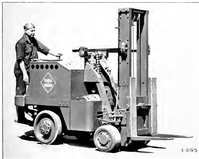
The new Elwell-Parker 6000 pounds capacity elevator chisel truck.
